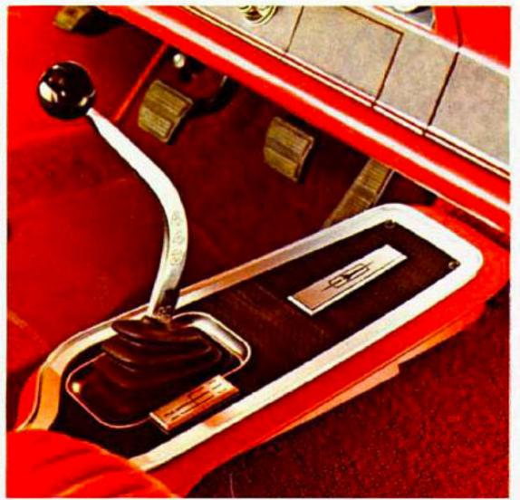
Knob hill. Classy Hurst shifter takes root in 4-4-2's nifty, optional sports console. 4-speed fully synchronized manual (shown) or 3-speed Turbo Hydra-Matic 400 at extra cost. A floor-mounted, fully synchronized, heavy-duty 3-speed manual, standard. And away you go!
