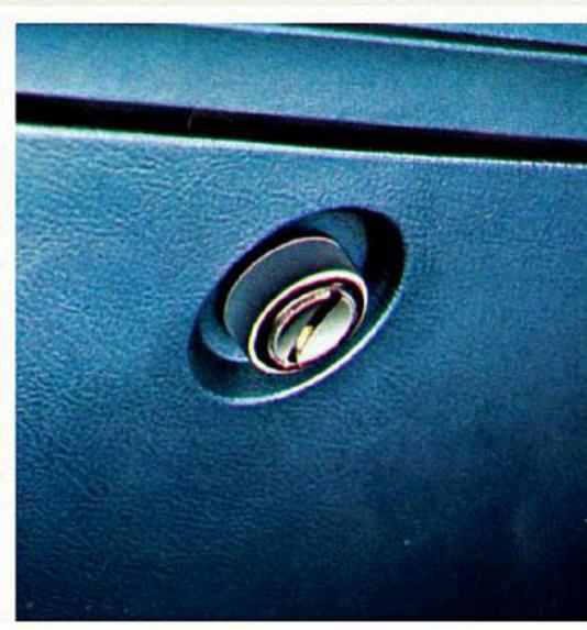
But, you don't want pushbuttons everywhere. So we replaced the one on the glove compartment door with a new lockable, easy-open, easy-close rotary latch. The compartment, incidentally, is deeper and will take on a lot more paraphernalia this year.
