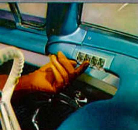
**All-Electric Power Window Lifts** on the '57 Oldsmobile raise and lower windows at the touch of a finger. There are separate controls for each window with the master control located in a convenient position . . . to the left of the instrument panel.
