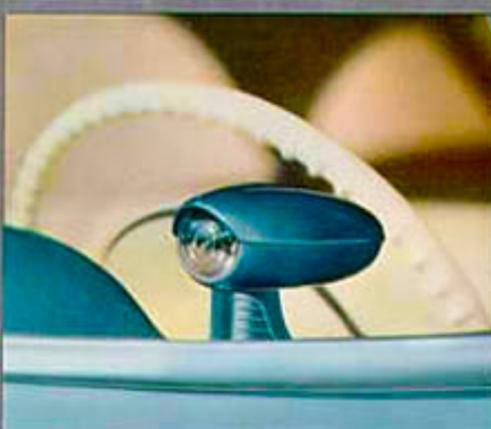
**Oldsmobile's Autronic-Eye** automatically dims your headlights when oncoming cars approach, then switches them back to bright when traffic has cleared. Saves you up to 200 "steps" an hour in average highway driving. An over-ride permits manual control.
