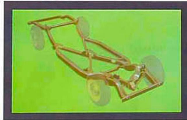
**New Extra-Wide Frame** takes a new shape for greater sturdiness and resistance to weaving and twisting. This frame is of much heavier construction and is full 8 inches wider on all Oldsmobile series, providing a broad base for smoother cornering, steadier handling, more solid body mounting. Deep-channel, "I-beam X-member" design adds the final touch of rugged strength and stability to an all-new Oldsmobile engineering masterpiece.
