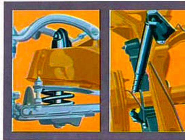
**New Pivot-Poise Front Suspension** features ball-and-socket pivots for easier steering, a wider spring base for increased stability. **Redesigned rear suspension** puts shock absorbers outside rear springs for a firmer, better-balanced, road-hugging ride.
