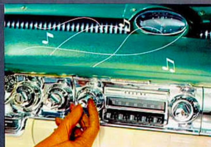
**Oldsmobile's De Luxe Radio** provides simple volume and bass-treble controls . . . a handy push-button selector for finger-tip tuning . . . and powerful six-tube, full-fidelity reception. Front speaker is centrally located beneath the opening at the base of the Span-A-Ramic Windshield, which acts as a sound reflector.
