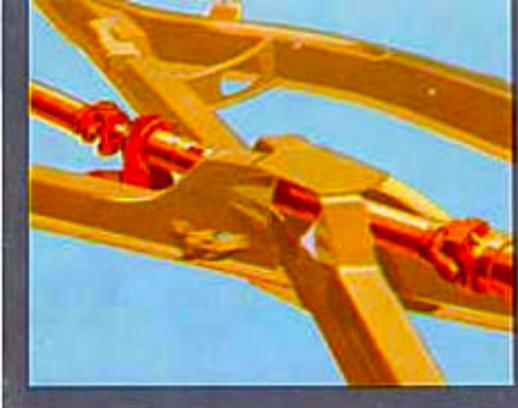
**New L-Bow Propeller Shaft** . . . the secret of Oldsmobile's new low look! Two-piece, three-joint construction permits a lower center of gravity and eliminates whip and vibration.
