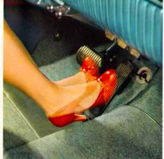
NEW PEDAL-EASE POWER BRAKES Like magic, Oldsmobile's Pedal-Ease Power Brakes turn "foot-weight" pressure into dynamic stopping power. With almost identical-height brake and accelerator, you swing from "go" to "stop" without lifting your heel. Your heel is cradled in a new rest packet to prevent slipping. Braking vacuum power is retained by a special valve when engine is
