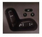
Both front seats feature 8-way power adjustment. The driver's seat features dual memory controls for a personalized fit at the touch of a button.
