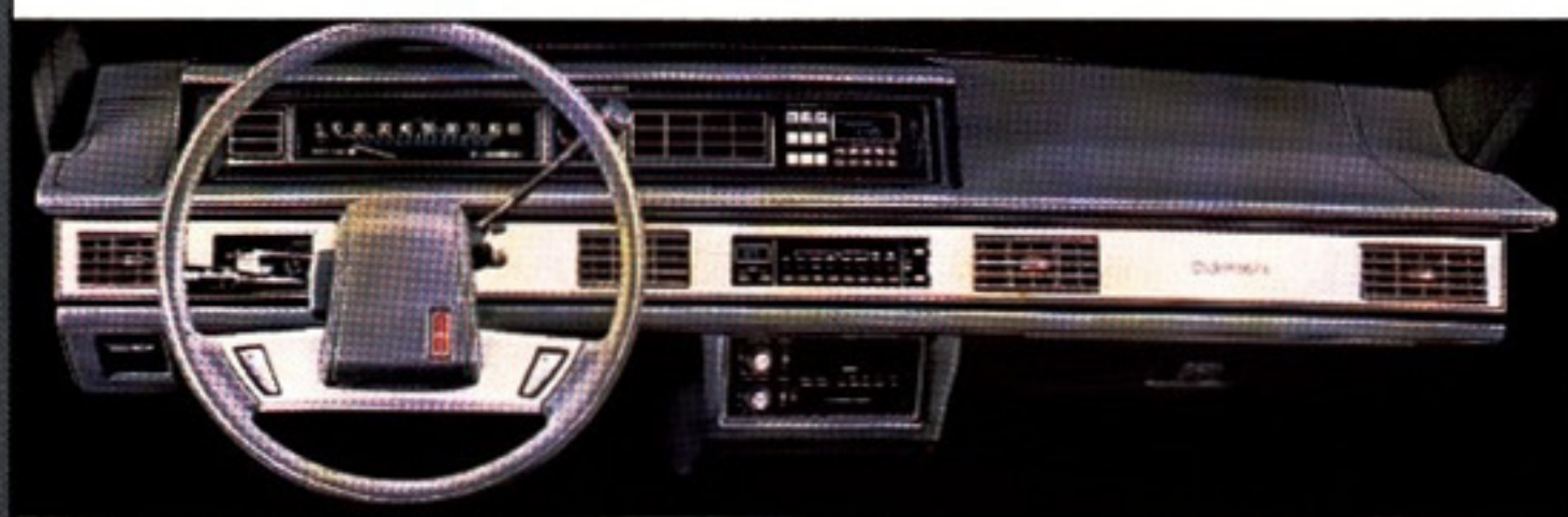
Delta 88 Royale instrument panel shown with available equipment.* *Note: Speedometers in Canada have major scale in km/h. Secondary in MPH and odometer in kilometres.
